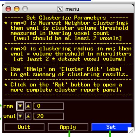
Press one of these buttons to create clusterized volume for display as new Overlay
